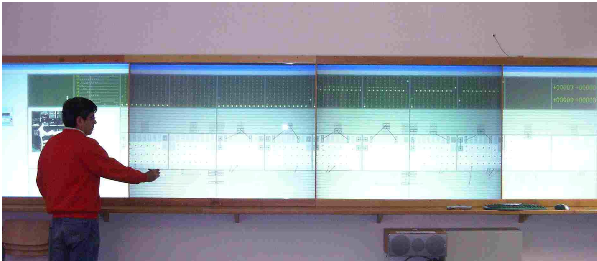
Figure 11: The ENIAC simulation running in the touch sensitive data wall installed in the Department of Mathematics and Computer Science, Freie Universität Berlin. The wall is six meters long and can display up to eight ENIAC units simultaneously.
